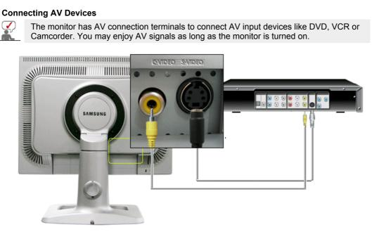
1. Input devices such as DVD, VCR or Camcorder are connected to the C-Video or S-Video terminal of the monitor using the C-Video or S-Video cable.
